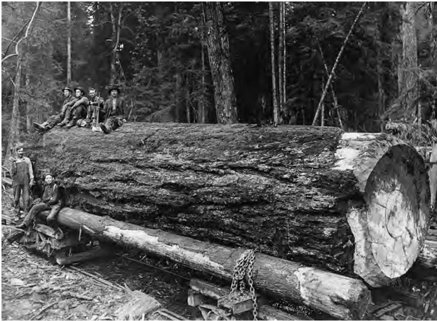
Loggers in the State of Washington, 1912 It took the sweat and skill of many men to conquer a giant Douglas fir like this one. An ax-wielding “sniper” had rounded the edges of this log so that a team of oxen, driven by a “bullwhacker,” could more easily drag it out of the woods along a “skid road.” Skid road (sometimes corrupted as skid row ) was also a name for the often-sleazy sections of logging towns, where loggers spent their time in the off-season.
